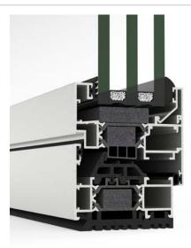
This 70 mm frame depth hinged system offers great thermal and acoustic performance combined with very simple fabrication, which is why it has become one of the most demanded series for aluminium windows, doors and balconies.
